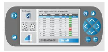
The CTR 9 records weld data and generates reports during the repair process. Print the report to testify to the quality of the welding and increase the trust in your body
